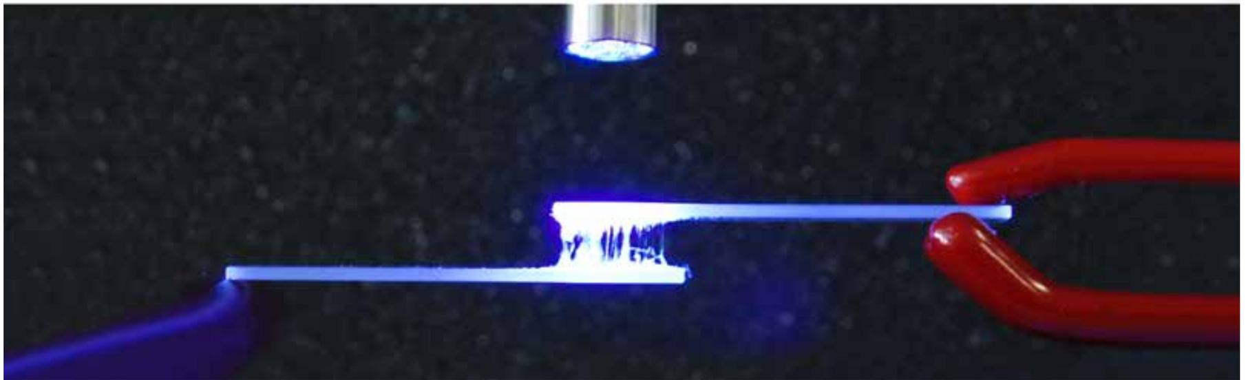
Visualizing the light-induced debonding feature of the supramolecular polymers used by AMI researchers. Under ambient conditions, the materials are powerful adhesives (top), whereas they liquefy and lose their adhesive properties upon heating or irradiation with ultraviolet light (bottom) (pictures: C. Heinzmann).
